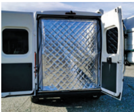
Insulation with multi-layers
